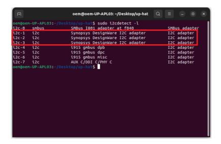
Test the Synopsys DesignWare I2C adapter (replace [I2CBUS] with the specific bus number identified from the previous command):
