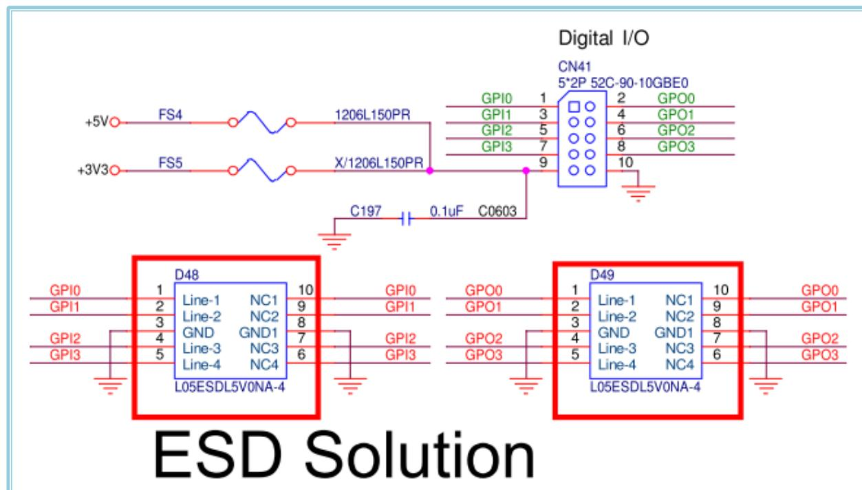
Note : (1) TVS placement must be close to Connector for ESD Solution .
