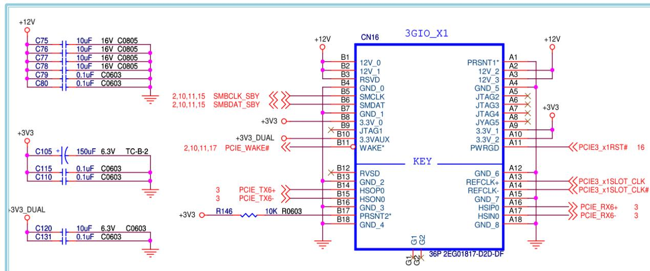
Figure 3-2 Mini-Card for mSATA / PCIE Switching Reference Schematic
