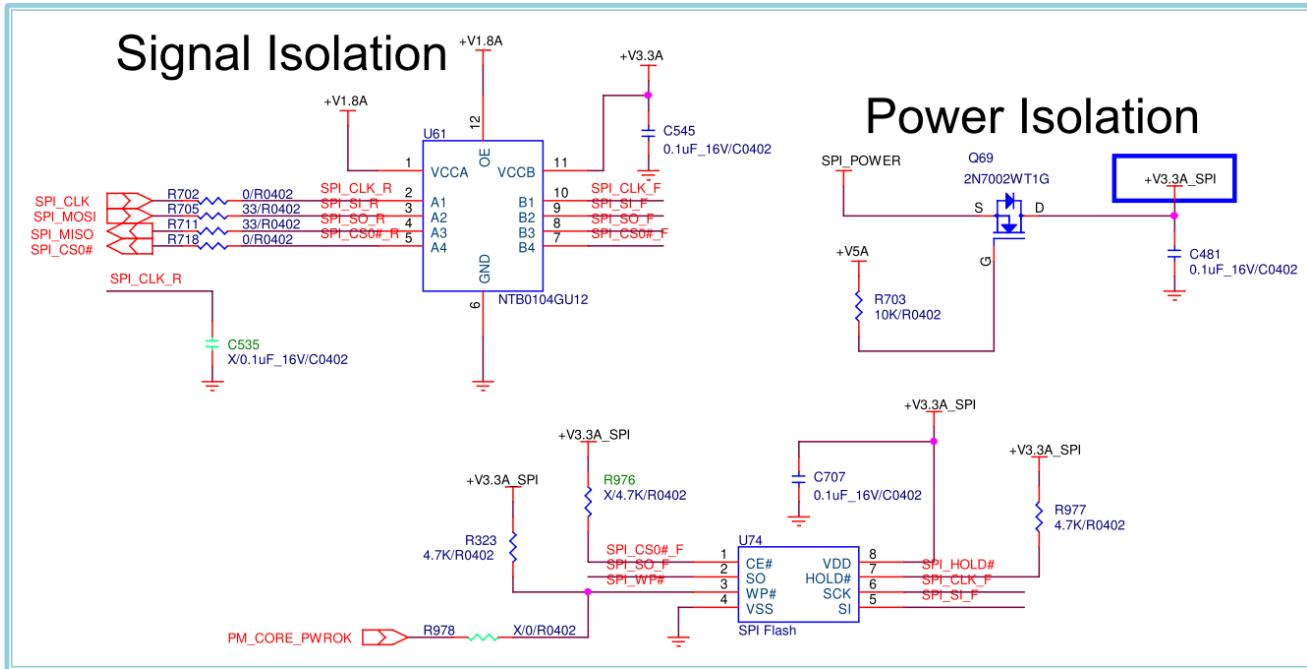
Note: SPI Signals must be added isolation circuit(level shift or N MOSFET) for System protection.
