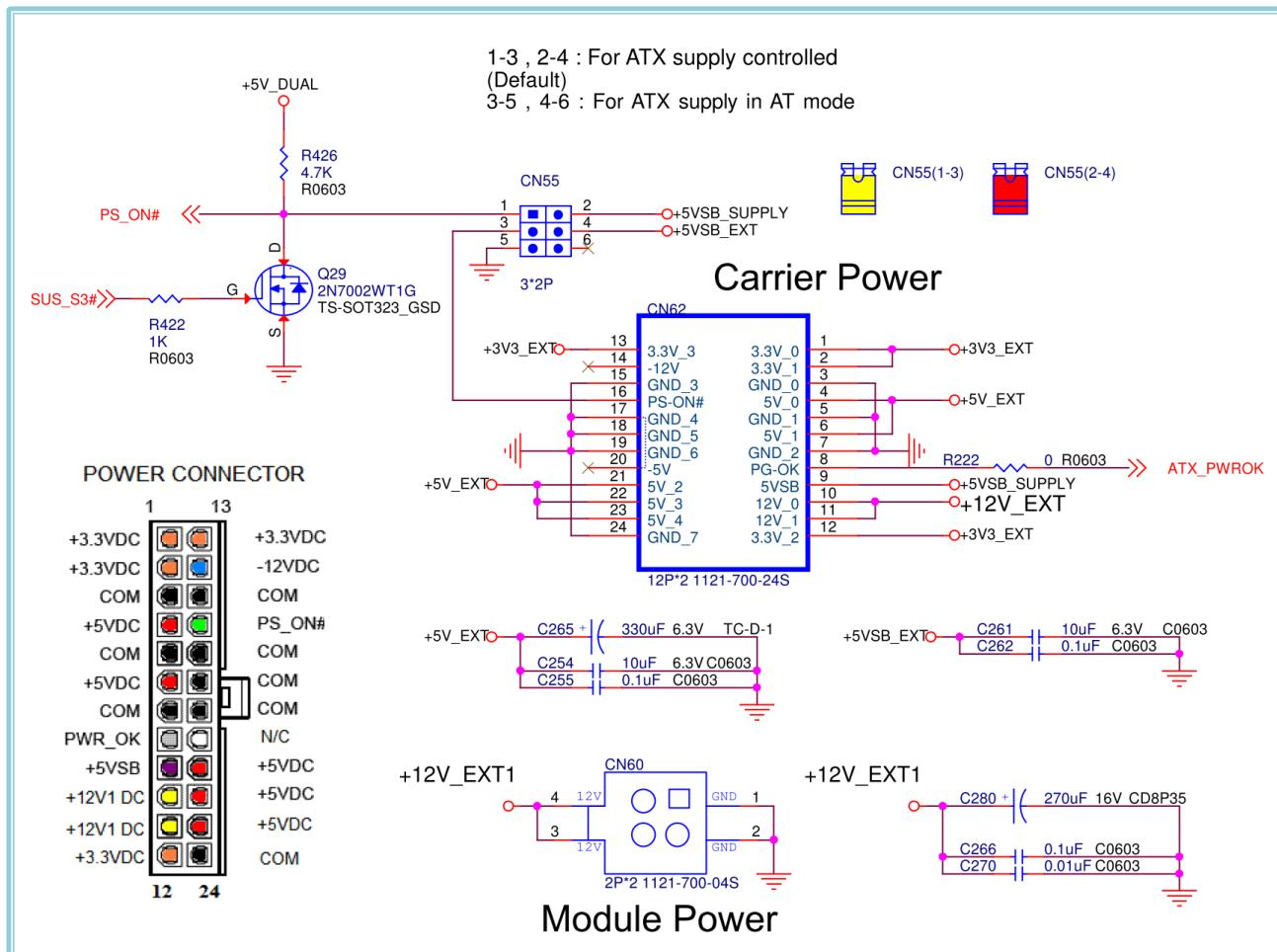
Note : Independent Power Input Design of COM Express Module Power Consumption Measurement Use.
