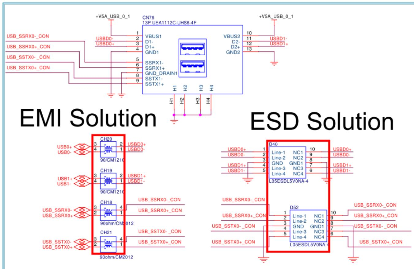
Note : TVS placement must be close to Connector for ESD Solution .
