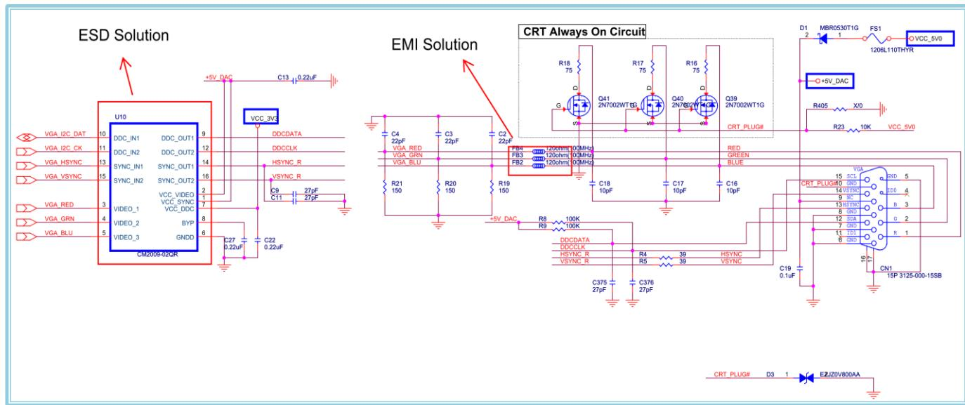
Note : CM2009 placement must be close to Connector for ESD Solution .
