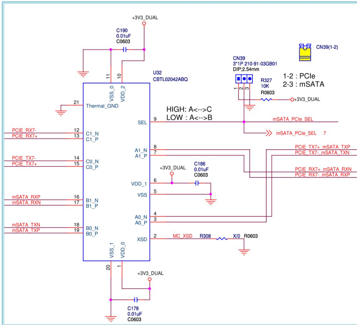
Figure 3-3 Mini-Card for mSATA / PCIE Reference Schematic
