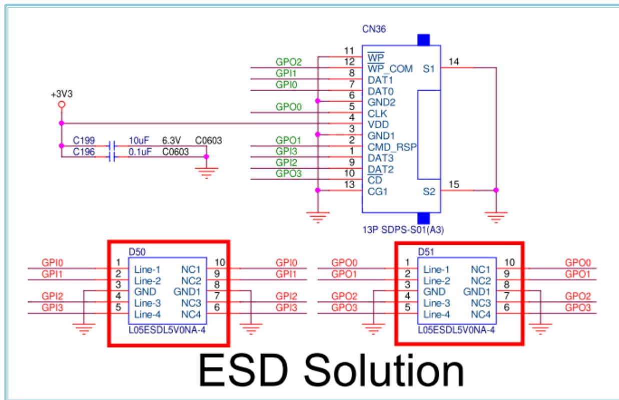
Note : (1) TVS placement must be close to Connector for ESD Solution .
