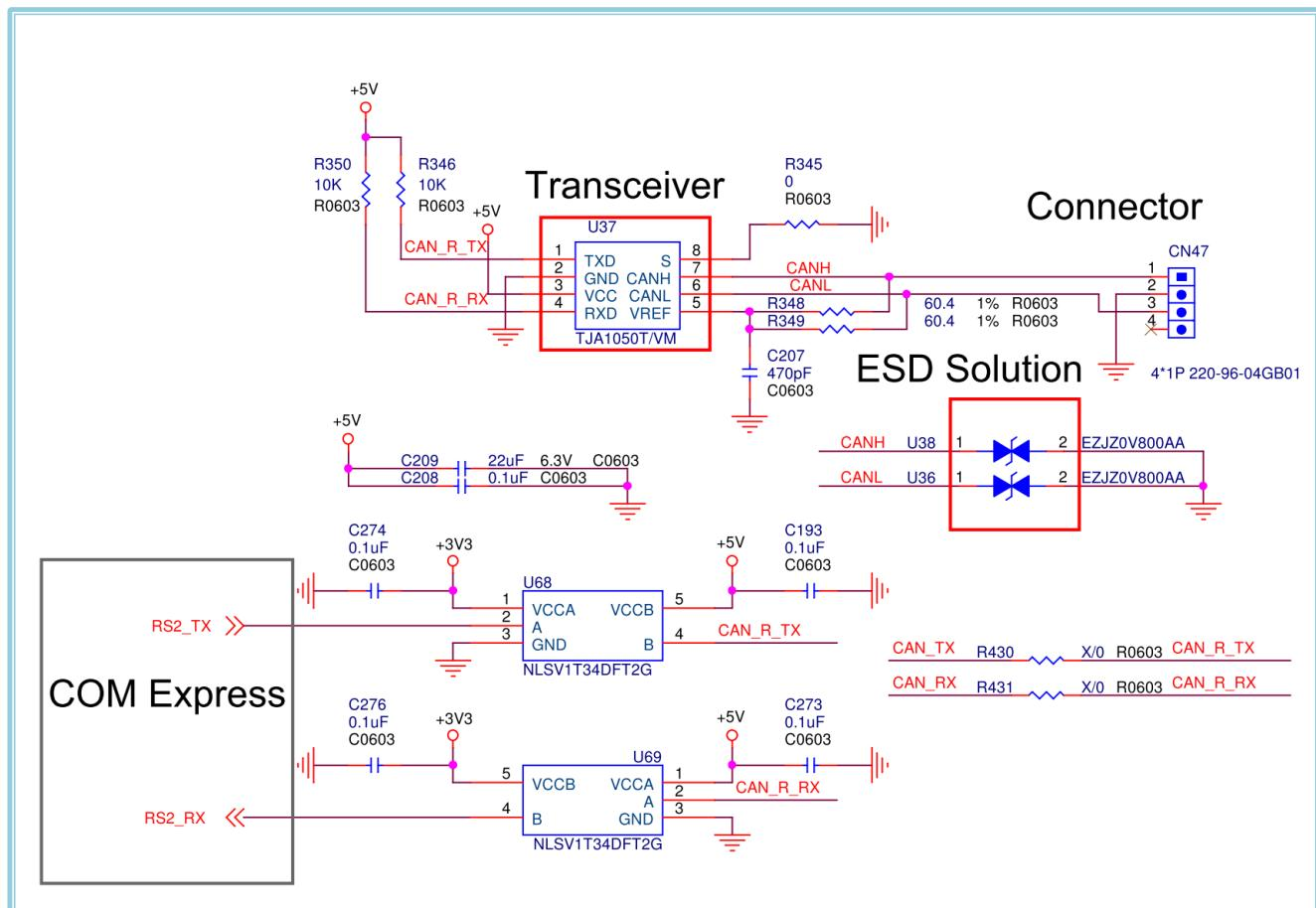
Note : VDR placement must be close to Connector for ESD Solution .
