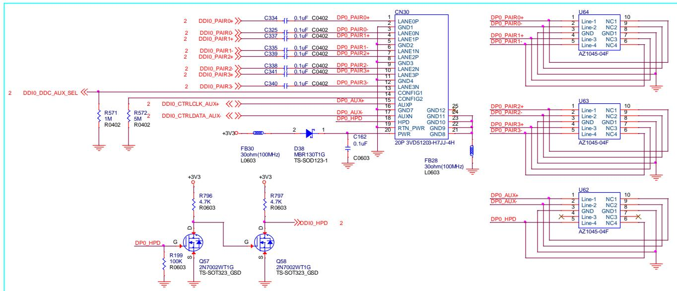
Note: TVS placement must be close to Connector for ESD Solution.
