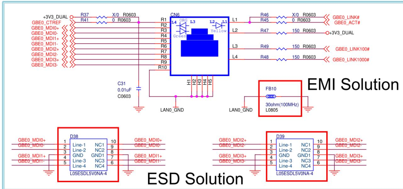
Note : TVS placement must be close to Connector for ESD Solution .
