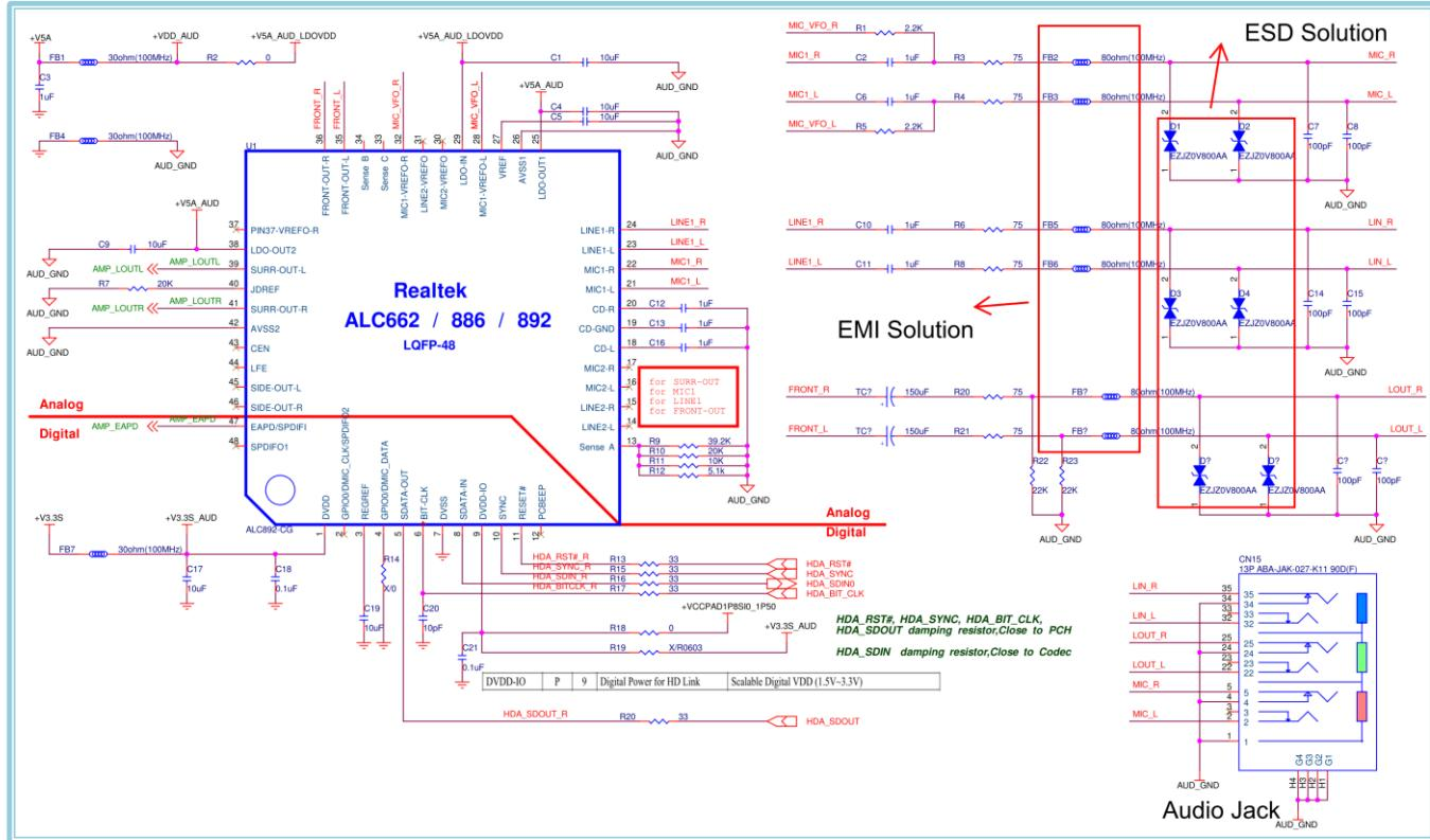
Note : VDR placement must be close to Connector for ESD Solution .
