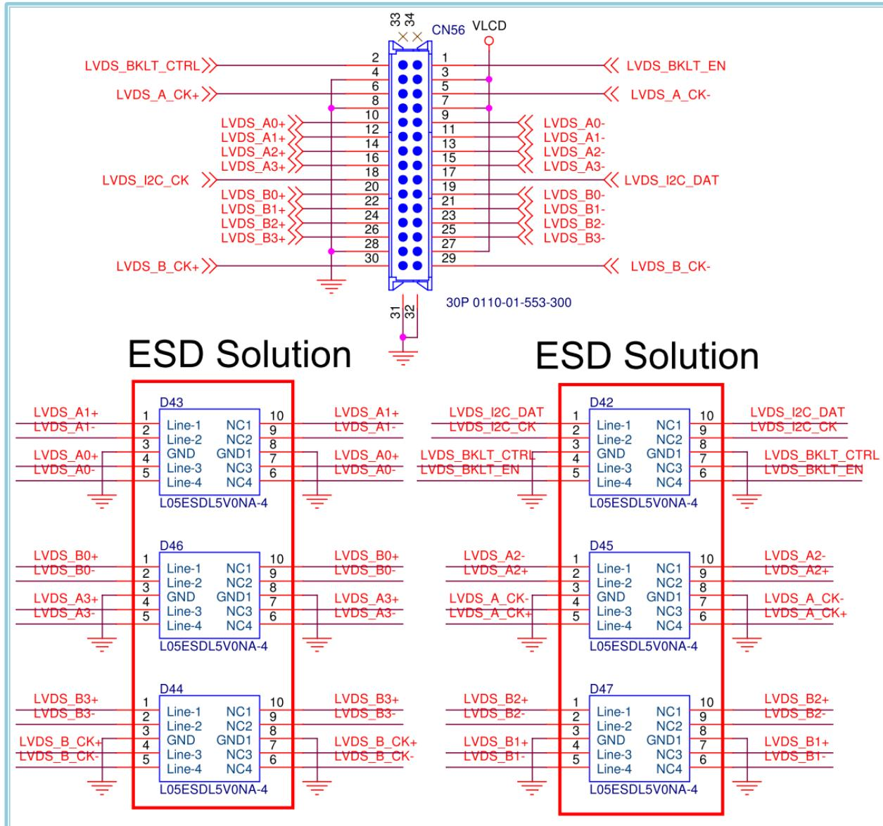
Note : TVS placement must be close to Connector for ESD Solution .
