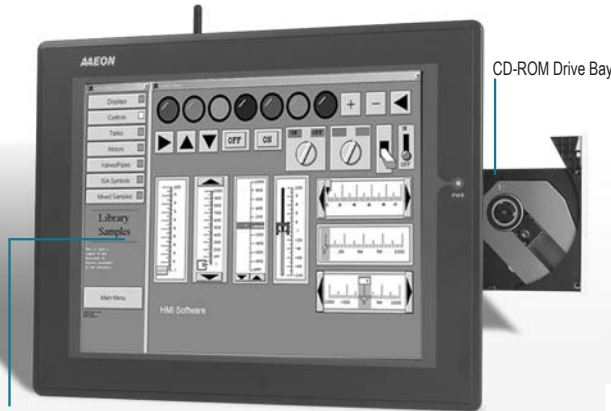
IP-65 certified front panel with touchscreen
