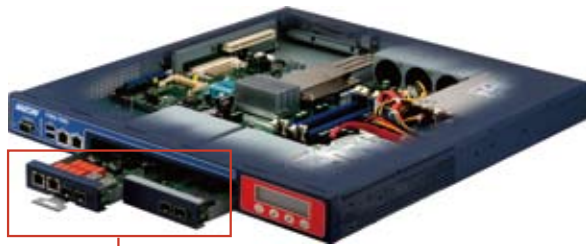
Modules could be two fiber modules or one fiber and one copper combination modules
